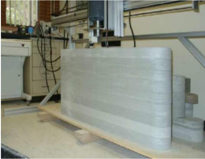
Figure 6.4 Concrete Slab from 3D Printer
